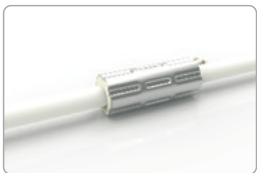
The anti-wicking ferrule is located at 115mm ( \pm 10\text{mm} tolerance) from the connector on the cable. For protection against water ingress from inside of cable wire and hence damage the light.
