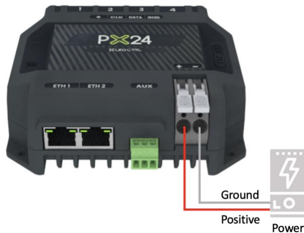
Figure 6 - PX24 Location of Power Input
